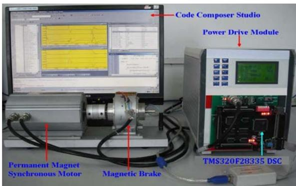
Fig. 3. Experimental setup of PMSM servo system.
