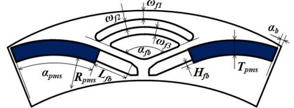
Fig. 5. Parameterization of the proposed IFVF-IPM rotor structure.
