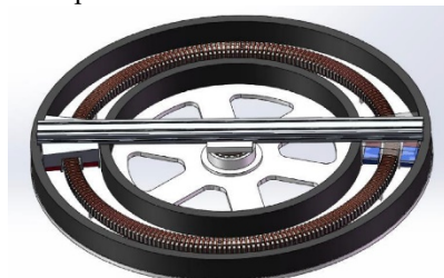
Fig. 3. Profile of the proposed TA-PMSLM.
